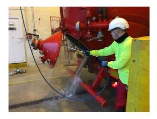
E78 Cleaning with high pressure water of fill- and discharge opening lids, rims included, lids and all joined parts
